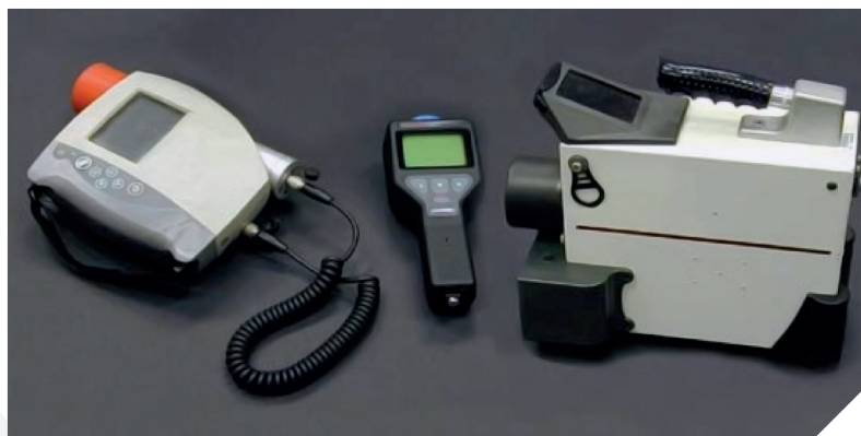
Typical handheld RIID detection systems; left to right: LaBr 3 (Ce), NaI(Tl), and HPGe. Reference: https://www.dhs.gov/sites/default/files/publications/RadiationDetectorsIdentifiers-TN_1009-508.pdf
