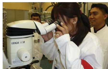
Examination of radioactively contaminated evidence by optical microscopy. The microscope is attached to a “glove-box” which allows the safe handling of radioactive material.
