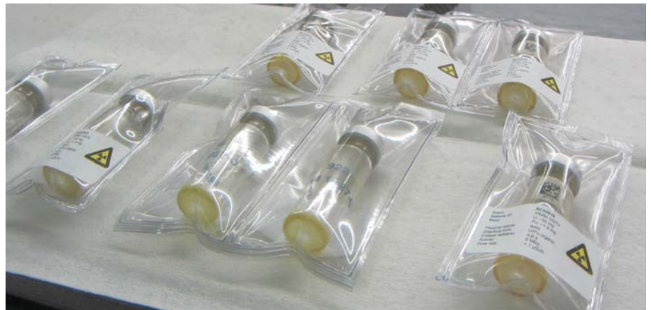
JRC-IRMM Large Sized Dried spikes are applied to measure the uranium and plutonium content of dissolved fuel solutions using isotope dilution mass-spectrometry. They are a fundamental part of the fissile material control of irradiated nuclear fuel. JRC-IRMM was visited by BMWG in November 2012
