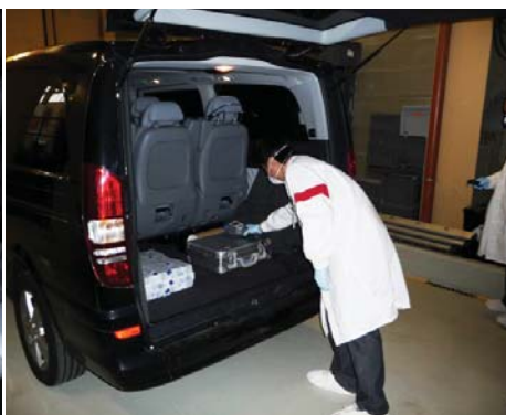
Exercises during the hands-on training on core capabilities in nuclear forensics. (Left) Prior to removing the evidence from the car, the dose rate of the object is determined enabling an initial assessment of the radiological safety. A first measurement is performed for the categorisation of the suspect material i.e. determining whether the material is a medical or industrial radioactive source, a naturally occurring radioactive material or a nuclear material. (Right) The team of specialists perform a “search and localise” exercise in order to verify the alleged illicit transport of radioactive material in a suspected vehicle.
