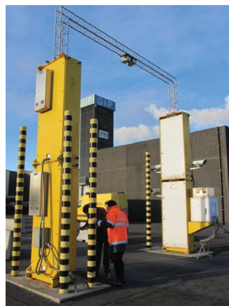
Vehicle radiation portal monitor at the Megaport of Antwerp visited during the BMWG meeting
