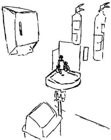
Figure 10. Hand wash basin – poor example (too small and too cramped)
