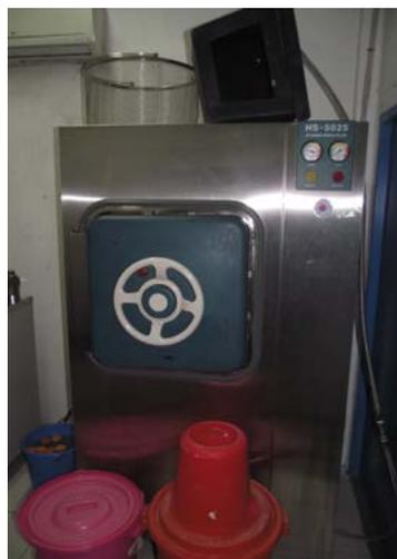
Figure 17. Barrier autoclave (unload side view)
