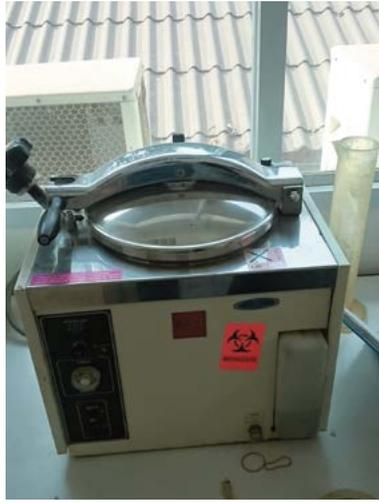
Figure 7. Bench top electric autoclave
