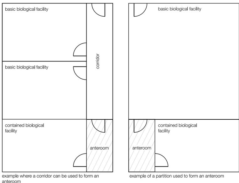
Figure 15. Examples of arrangement for separation of biological facilities
