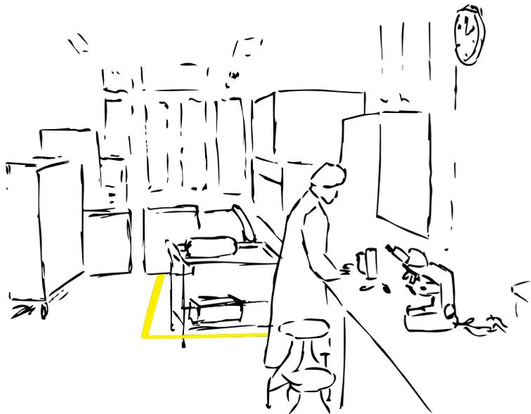
Figure 12. Example of safe zone around the BSC (indicated by yellow line)
