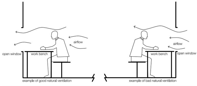
Figure 13. Examples of good and bad natural ventilation
