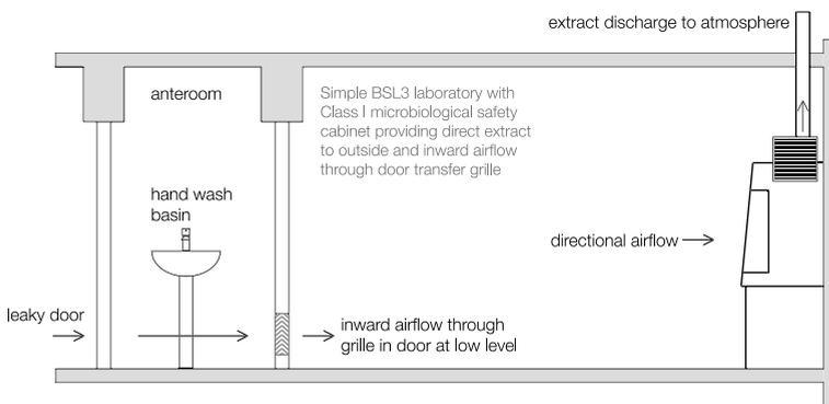
Figure 19. BSL3 Ventilation and airflow example
