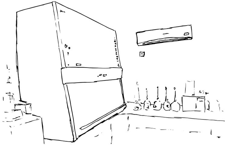
Figure 20. Ventilation: possible impact on safe BSC operation (Example 1)
