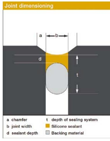
Figure 18. Joint dimensioning (Wacker Sealants - [www.wacker.com](http://www.wacker.com))
