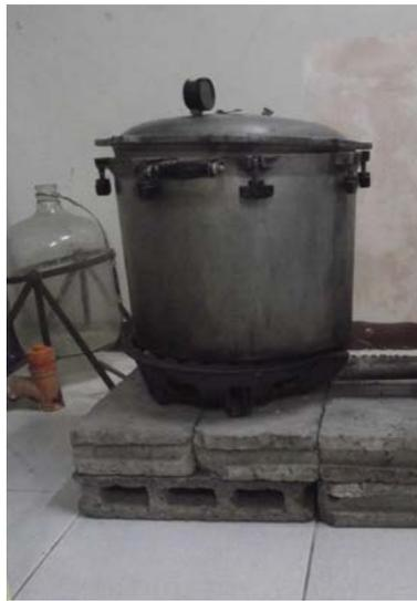
Figure 6. Gas heated pressure cooker type autoclave
