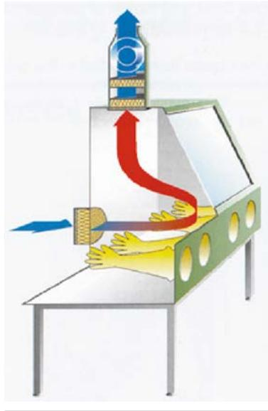
Figure 4. Class III Biosafety Cabinet
