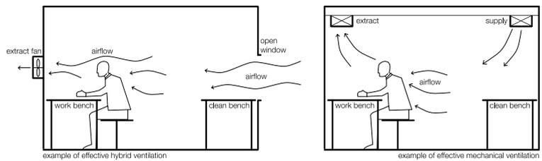
Figure 14. Examples of effective hybrid and mechanical ventilation
