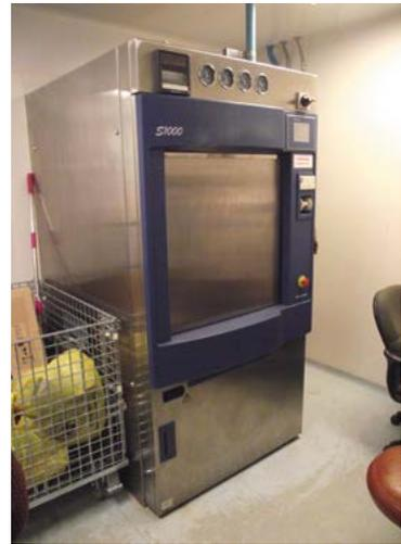
Figure 9. Large fixed floor mounted autoclave with automated loading door
