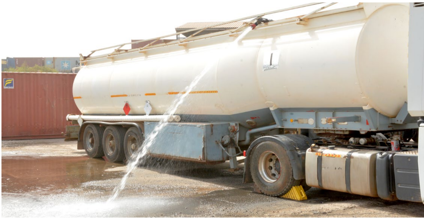
Leak of a toxic and flammable product.
