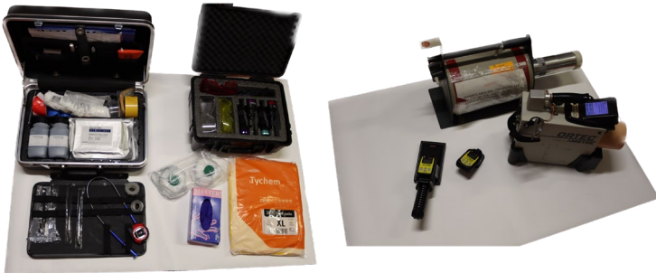
Figure 5-5. Image of conventional forensic tool (left) and radiation measurement equipment (right) provided by IFIN-HH.
