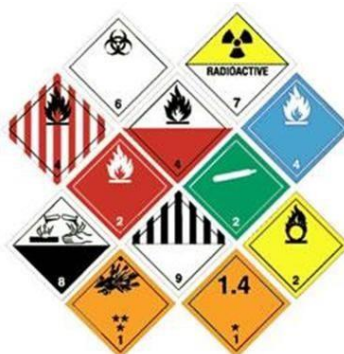
Fig. 1.3 UN Hazard Identifiers of the UN Committee on the Transport of Dangerous Goods by Road or Rail (ADR)
