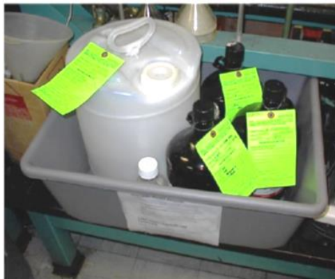
Fig. 3.3 Containers ready for pick-up, properly labelled and located in secondary confinement vessel
