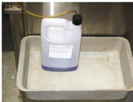
Fig. 3.2 Example of correct storage of mobile phase outflow from HPLC
