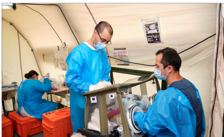
Two Uzbek laboratory experts process diagnostic patient samples in the Glovebox, a sub-pressurized workspace that allows the safe handling of samples with suspicion of risk group 4 pathogens.
